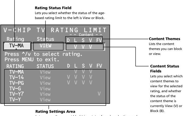
Lets you see the current block/view state of age-based ratings and associated content. The View (V) settings are coded in green, and the Block (B) settings are coded in red.
